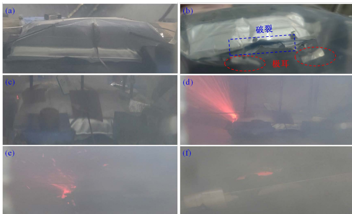
Figure 3. Experimental process for thermal runaway of pouch-type ternary lithium-ion battery 图 3. 软包锂电池热失控实验过程
