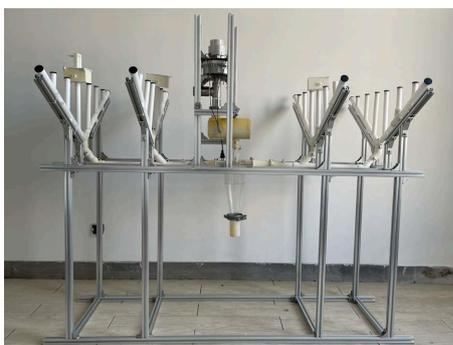
Figure 6. Experimental prototype of particle collecting device
