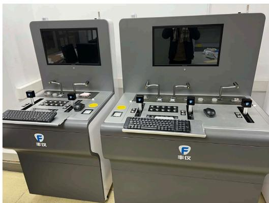
Figure 1. Automatic pressure gauge testing device
