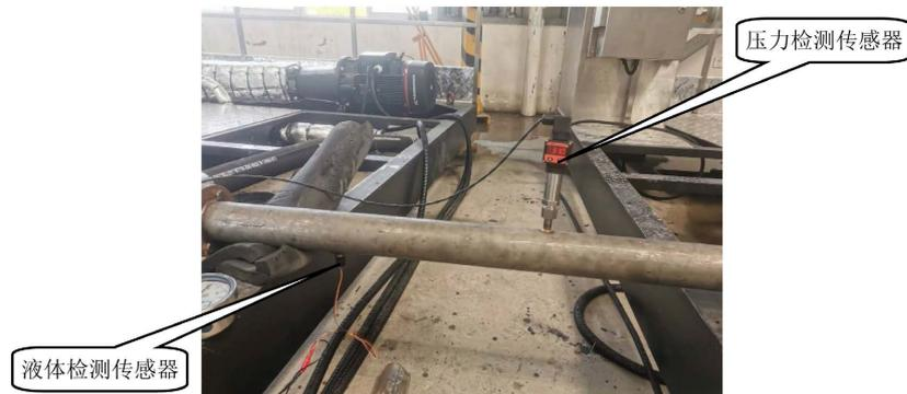
Figure 7. Detection sensor installation position diagram
