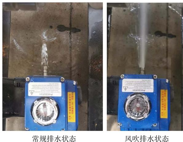
Figure 8. Comparison of drainage status of drainage valves
