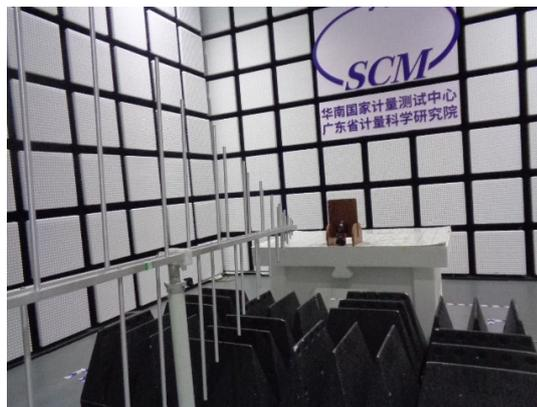
**Figure 4.** Laboratory of radio frequency electromagnetic field radiation immunity
