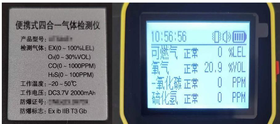
**Figure 2.** Some incorrect examples of nameplate (left) and display panel (Right)
