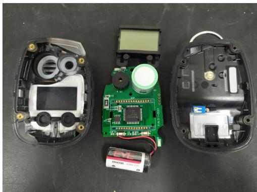
**Figure 1.** Internal structure of a certain model of hydrogen sulfide gas alarm detector
