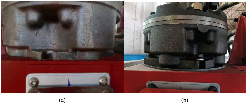
Figure 5. Installation and positioning of the anti-loosening structure. (a) Before installation; (b) After installation 图 5. 安装定位防松结构。(a) 安装前; (b) 安装后
