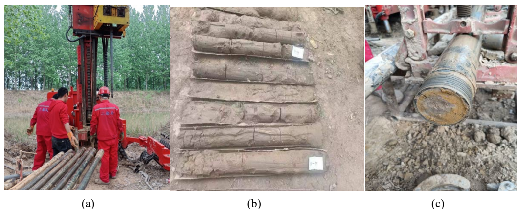
Figure 6. Field sampling. (a) Site drilling; (b) to obtain silt and clay samples; (c) to obtain sand samples 图 6. 现场取样。(a) 现场钻进；(b) 获取粉土、黏土样品；(c) 获取砂样
