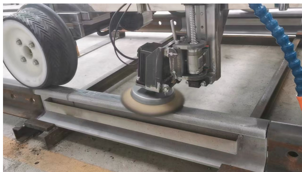
Figure 14. Railway track milling de-icing experiment
