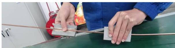
**Figure 2.** Current method of straightening
