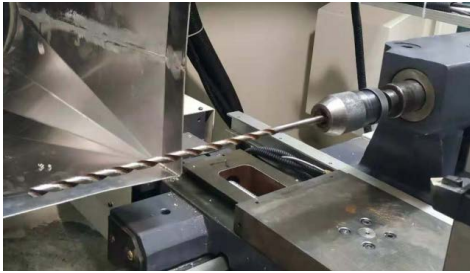
Figure 20. Restructured inner hole processing tail-stock
