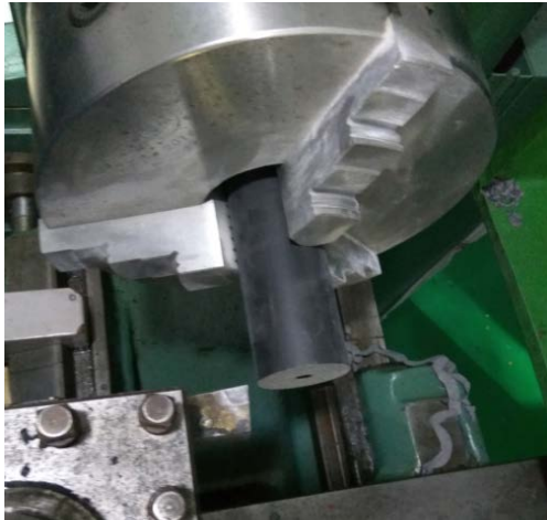
Figure 3. Outer circular end face of rough turning 图 3. 粗车外圆端面
