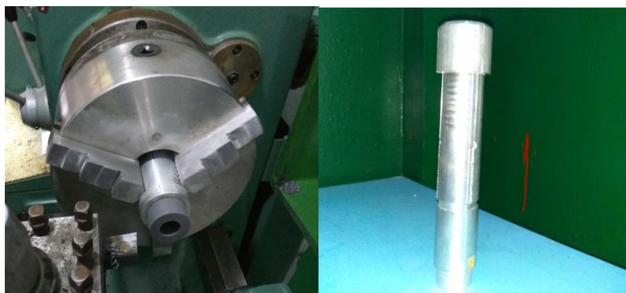
Figure 6. Finish outer circular end face and the rupture sleeve used in the sequence process
