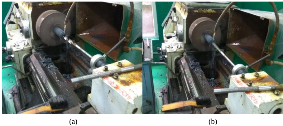
Figure 4. Drilling and reaming 图 4. 钻孔及铰孔
