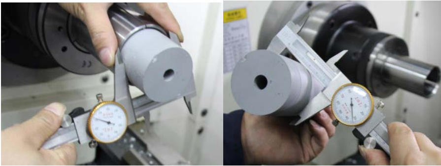
Figure 19. Verification of clamping force test 图 19. 夹持力试验验证
