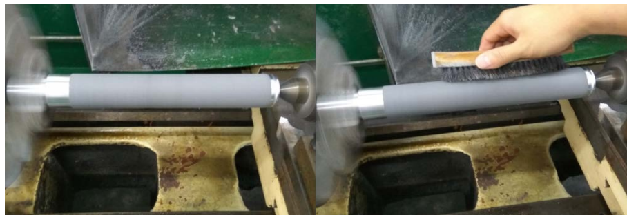
Figure 5. Finish outer circle and brush the residual powder of the grain 图 5. 精车外圆及刷残留的药柱粉末
