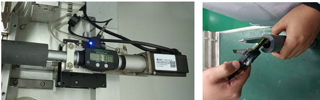
Figure 9. Determination test of tension required for inner diameter detection 图 9. 内径检测所需的涨紧力的确定试验
