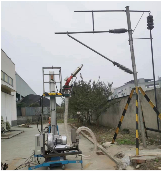
Figure 12. Site diagram of the prototype test of the hot air blowing device for contact line insulators 图 12. 接触网绝缘子热风吹扫装置样机试验现场图
