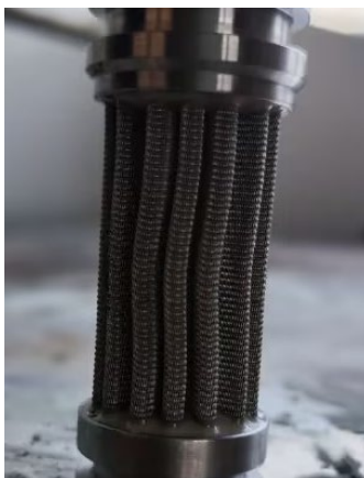
Figure 4. Picture of the new filter heating furnace after 3 min at 350℃ 图 4. 新过滤器加热炉 350℃保温 3 min 后图片
