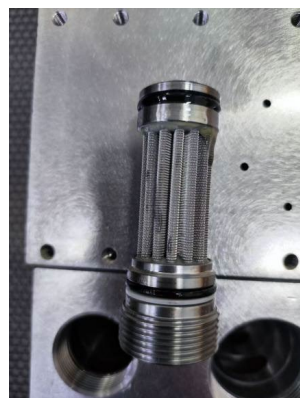
(b) Disassembly of new filters after assembly (b) 组装后拆解新过滤器
