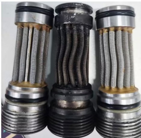
Figure 5. Return to the picture after the filter screen is heated 图 5. 返回过滤器滤网加热后图片
