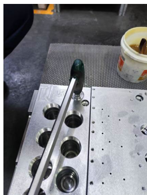
(a) Assembly of new filters (a) 新过滤器组装
