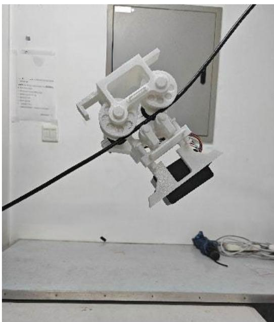
Figure 12. Walking test of arc sag detection robot
