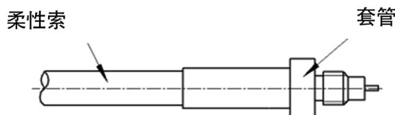
Figure 1. Assembly schematic of flexible rope sleeve module
