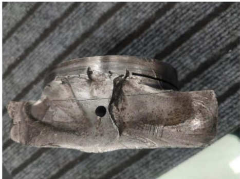
Figure 7. Macro-morphology of convex shaft fracture 图 7. 凸轴断口宏观形貌
