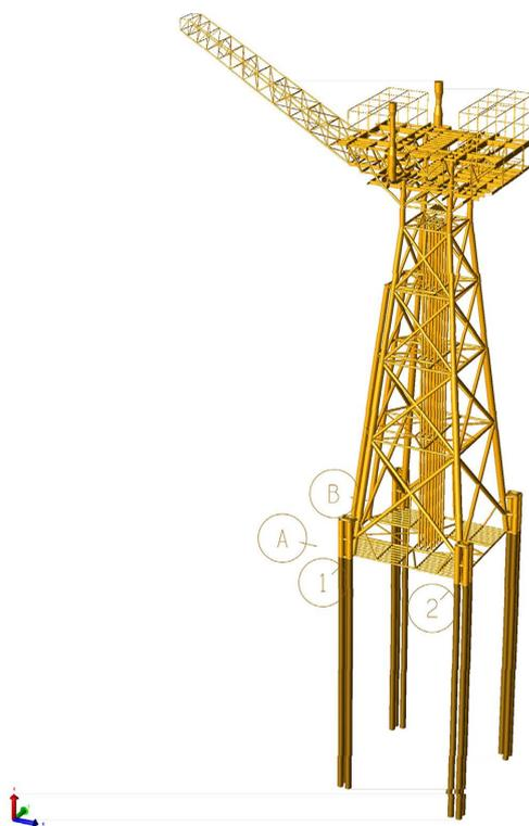
Figure 1. Jacket-and-gantry-platform model
