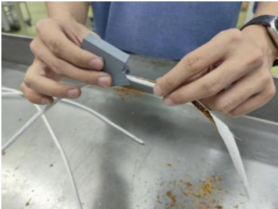
Figure 1. Blade-type cigarette cutting experiment 图 1. 刀片式划烟刀切割实验
