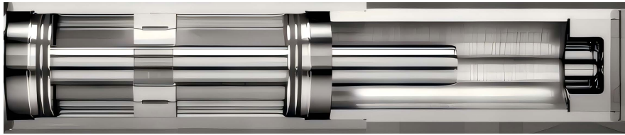
Figure 2. Internal structure diagram of double-rod hybrid energy-dissipative viscous damper 图2. 双出杆混合耗能式黏滞阻尼器内部构造图 ②
