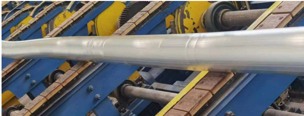
Figure 6. Bamboo-like defects 图 6. 竹节状缺陷
