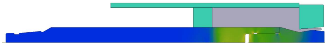
Figure 11. Stress in the needle and needle tip 1 s after the start of backward displacement of the optimized perforator 图 11. 优化后穿孔针向后变位开始后 1 s 时针和针尖的应力
