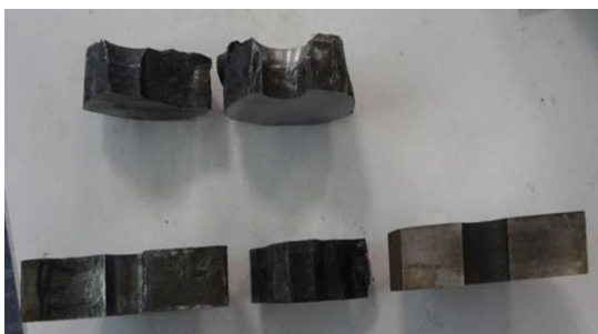
Figure 5. Fracture surface of roller sample 图 5. 滚子切样断口图
