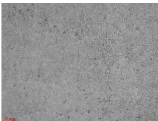
Figure 12. Microstructure of the surface layer of roller No. 3 magnified 500 times 图 12. 放大 500 倍 3 号滚子表层组织
