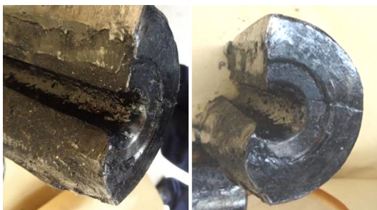
Figure 4. Damage to rolling elements 图 4. 滚动体损坏
