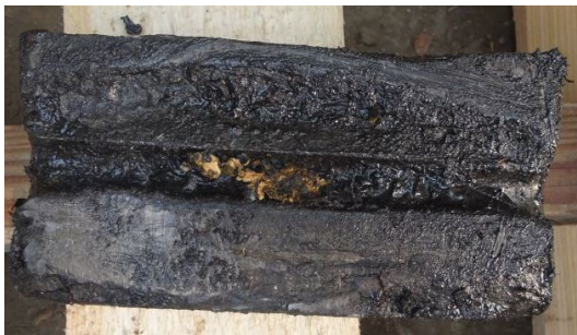
Figure 2. Damage image of 1# rolling element 图 2. 1#滚动体损坏图
