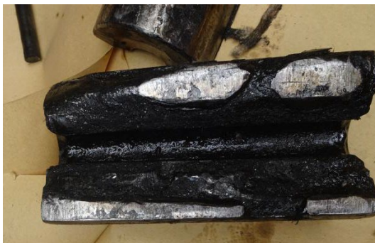
Figure 3. Damage image of 2# rolling element 图 3. 2#滚动体损坏图
