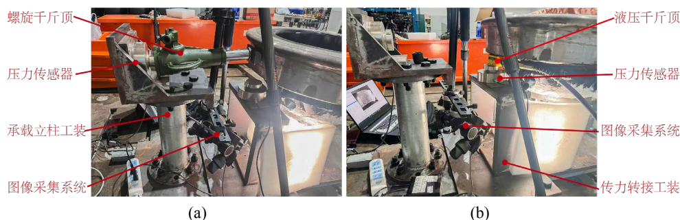
Figure 2. Experimental setup: (a) vertical loading; (b) lateral loading 图 2. 现场试验图: (a) 垂向载荷加载; (b) 横向载荷加载
