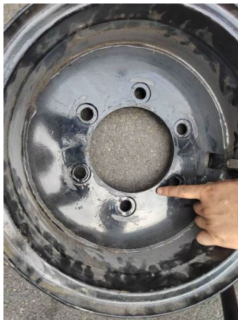
Figure 2. Hub deformation diagram
