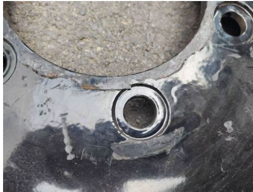
Figure 3. Hub wear detail diagram 图 3. 轮毂磨损细节图
