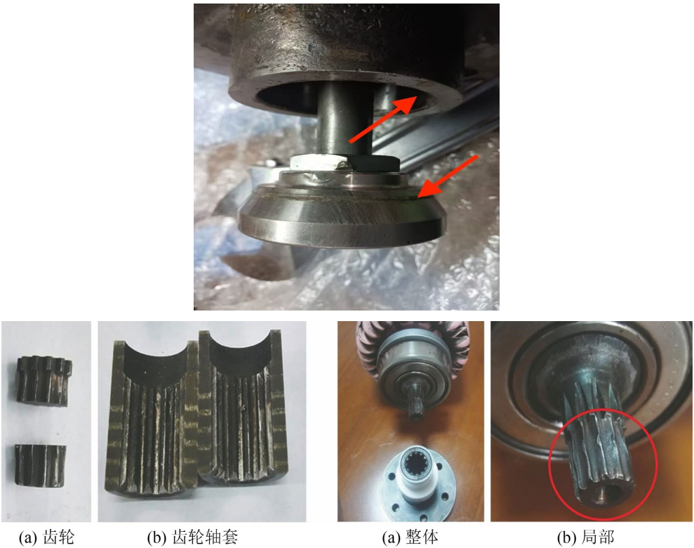
Figure 1. Severe mechanical damage (gear tooth breakage, bracket fracture)
