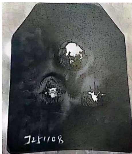
Figure 3. JC251108 (after the experiment) 图 3. 大号插板 JC251108 (实验后)
