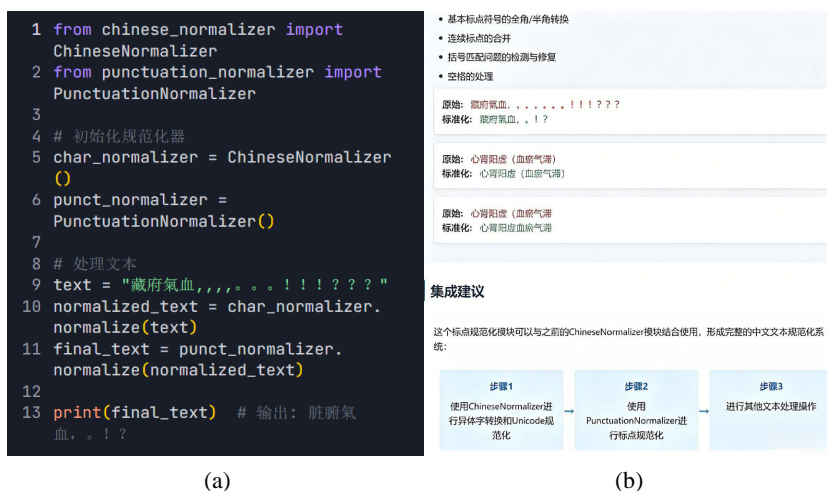
Figure 2. Trae-based punctuation normalization code and visualization interface 图 2. Trae 标点符号规范化代码及可视化界面
