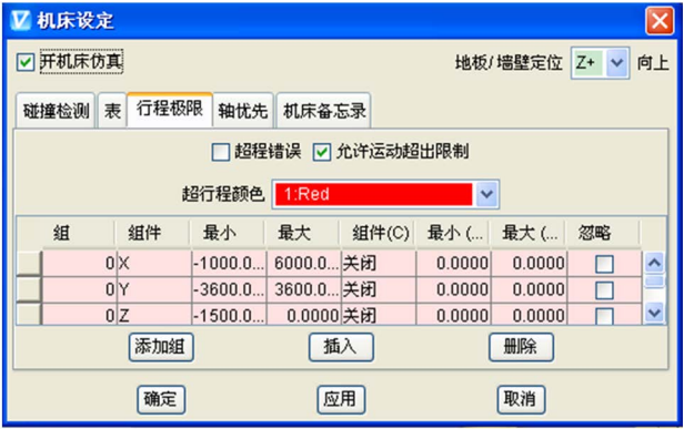
Figure 3. The setting of machine processing range 图 3. 机床行程设置
