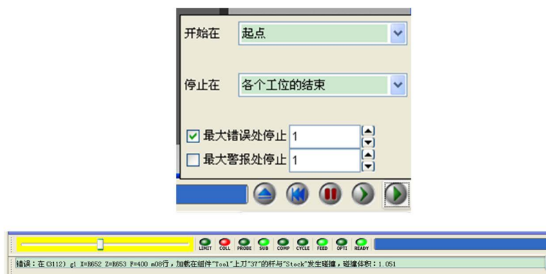
Figure 10. The function of simulation pause 图 10. 暂停示意
