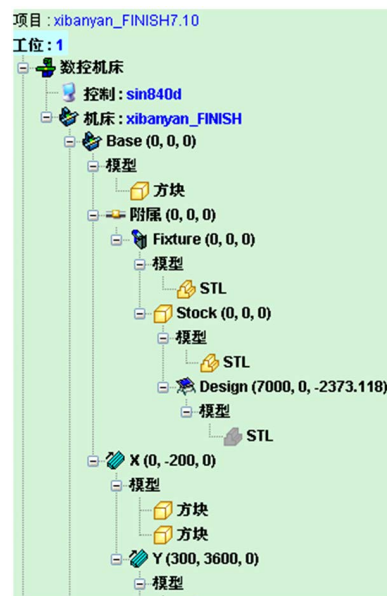
Figure 1. The topology structure of parts 图 1. 组件拓扑结构
