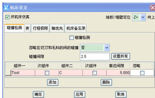
Figure 8. The setting of collision 图 8. 碰撞设置
