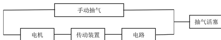
Figure 1. Logic diagram of each component of 04A Chemical agent detector kit
