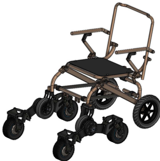
Figure 4. Assembly diagram of the obstacle-crossing add-on mechanism structure 图 4. 越障附加机构结构装配图
