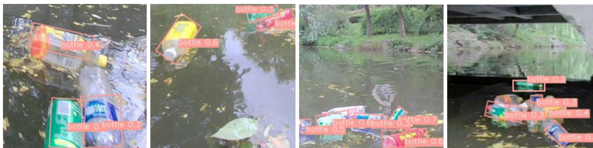
Figure 8. Results of rotating target detection of water garbage
