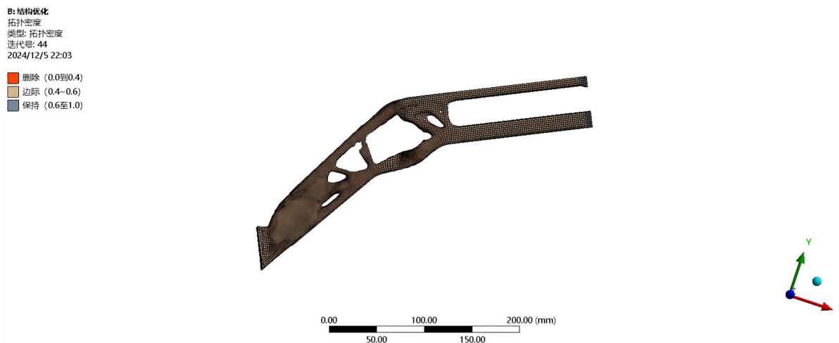
Figure 8. Topology optimization result 图 8. 拓扑优化结果
