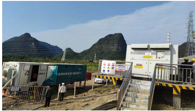
Figure 2. High and low voltage ride through test wiring and on-site testing diagram
