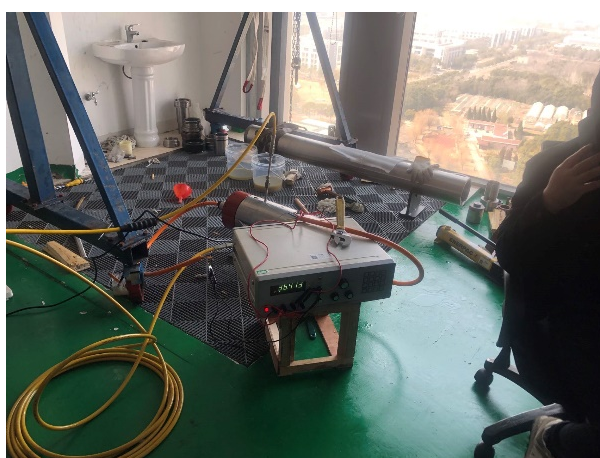
Figure 19. Contact resistance measurement after 25 wet insertions
