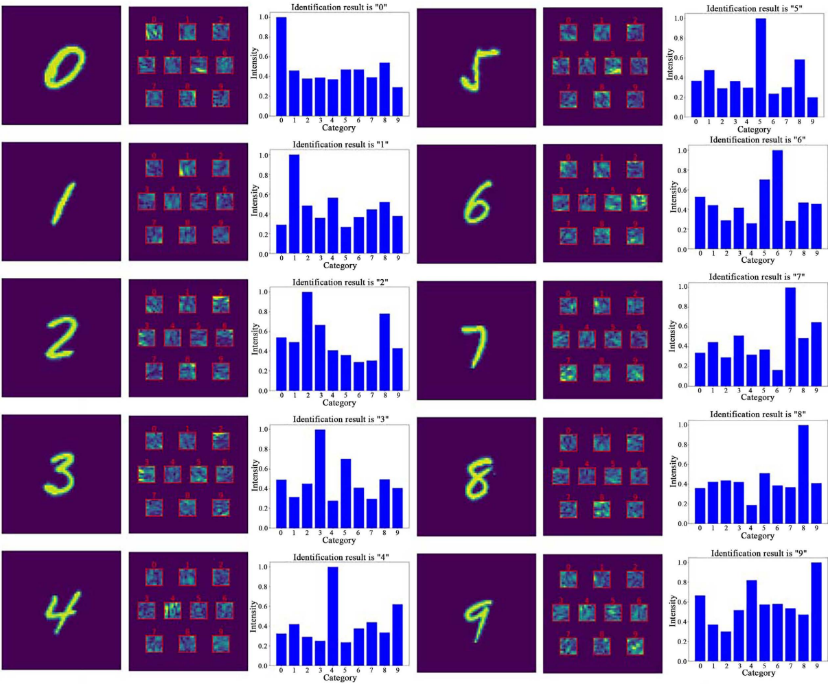
Figure 6. Energy distribution of the nonlinear D 2 NN for the recognition of ten handwritten digits 0~9 with 64 × 64 neurons 图 6. 64 × 64 神经元数量下非线性 D 2 NN 对 0~9 十个手写数字识别的能量分布图
