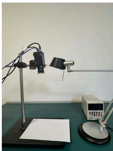
Figure 1. Multispectral image acquisition platform
