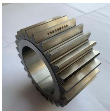
Figure 3. Schematic diagram of pitting fault of planetary gear
