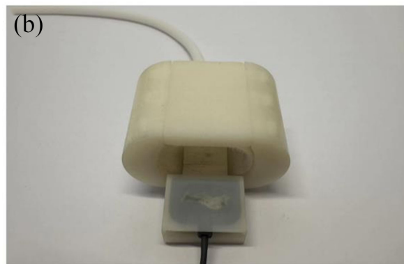
Figure 14. 3D structure diagram and physical diagram of piezoelectric sensing finger sleeve
