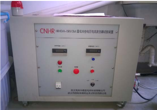
Figure 3. Lightning impulse voltage and current generator test device 图 3. 雷电冲击电压电流发生器试验装置
