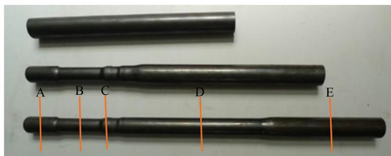
**Figure 9.** Hardness testing location of rotary forging shaft
