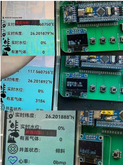
Figure 4. Physical object diagram of the display data test for the display module 图 4. 显示模块显示数据测试实物图
