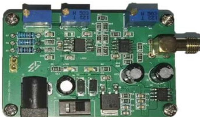
**Figure 11.** Signal conditioning hardware circuit physical diagram
