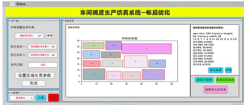
Figure 23. Layout diagram generated by genetic algorithm
