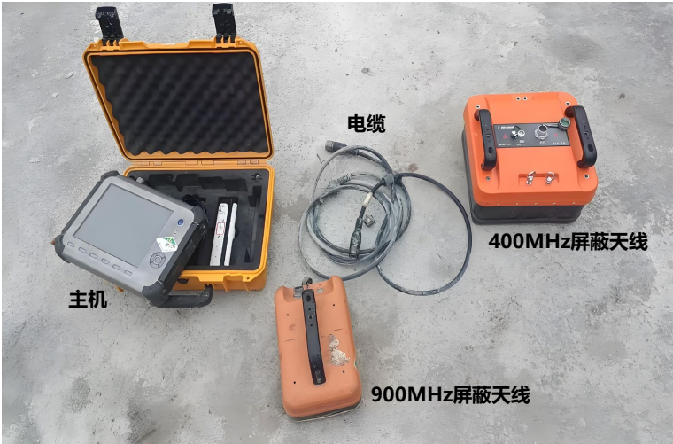
Figure 13. Component diagram of the LTD-2600 model ground penetrating radar 图 13. LTD-2600 型号探地雷达组成器件图
