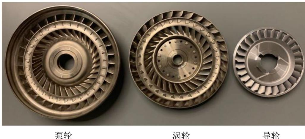
**Figure 14.** Sample part of each impeller of the torque converter
