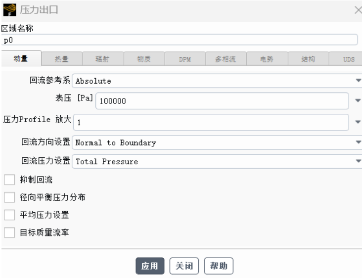
Figure 3. Boundary condition settings 图 3. 边界条件设置
