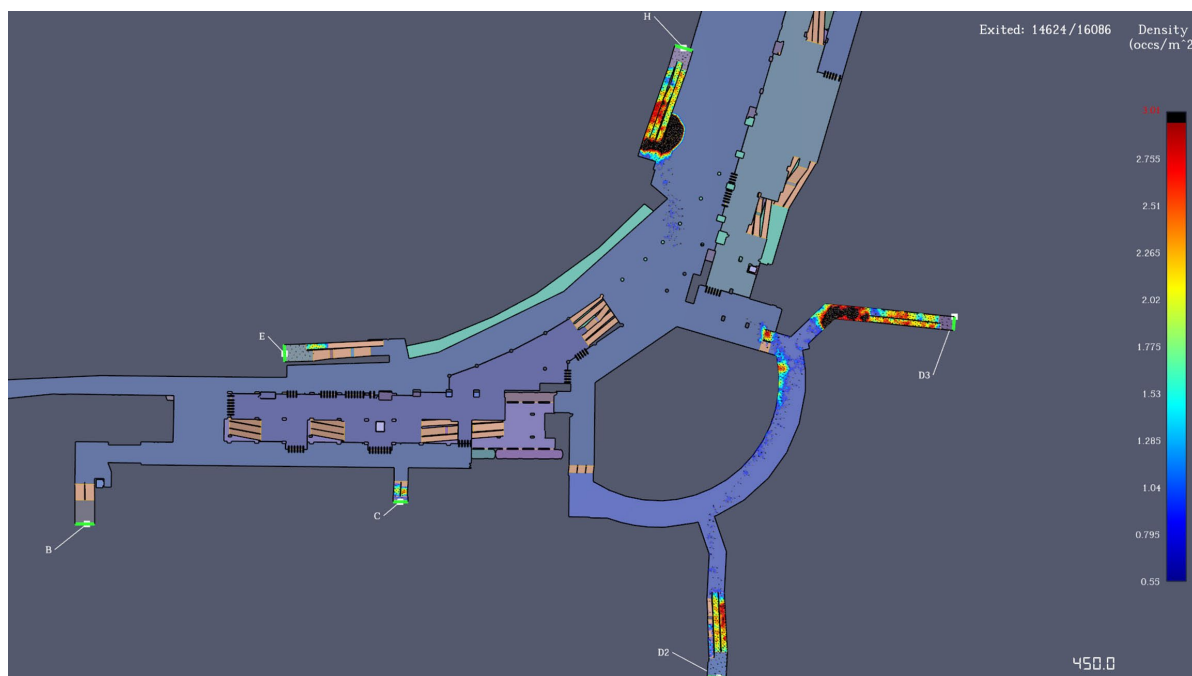
Figure 11. Diagram of crowd density at concourse layer during evacuation at 450 s
