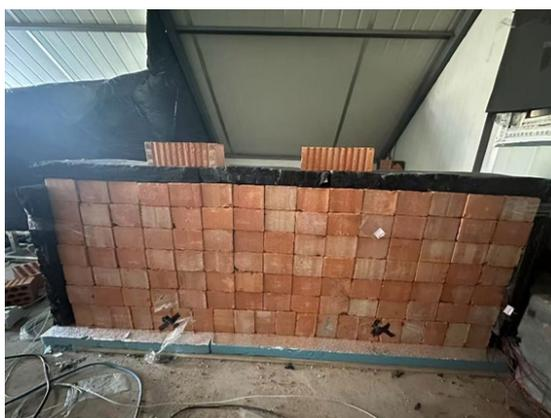
Figure 3. Real view of the heat storage wall sealed with thermal insulation at the top
