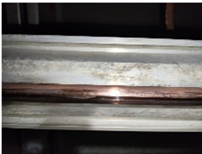
Figure 1. Contact wire abnormal wear diagram 图 1. 接触线异常磨损图
