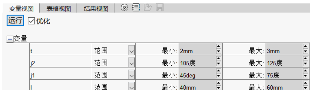
Figure 6. Setting optimization parameters in SolidWorks Simulation
