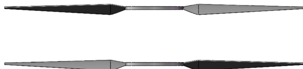
Figure 1. Geometric model of the fixed-pitch coaxial dual-rotor 图 1. 定桨距共轴双旋翼几何模型
