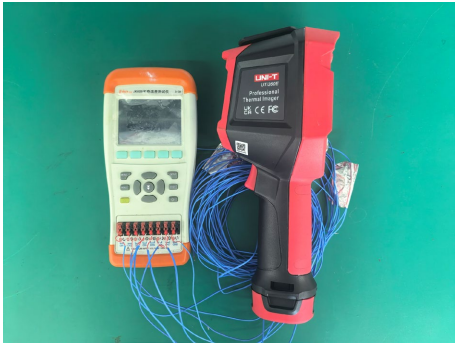
Figure 6. Temperature measurement instruments 图 6. 温度测量仪器
